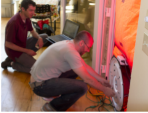
Blower door test – An essential tool for energy-efficiency audits
